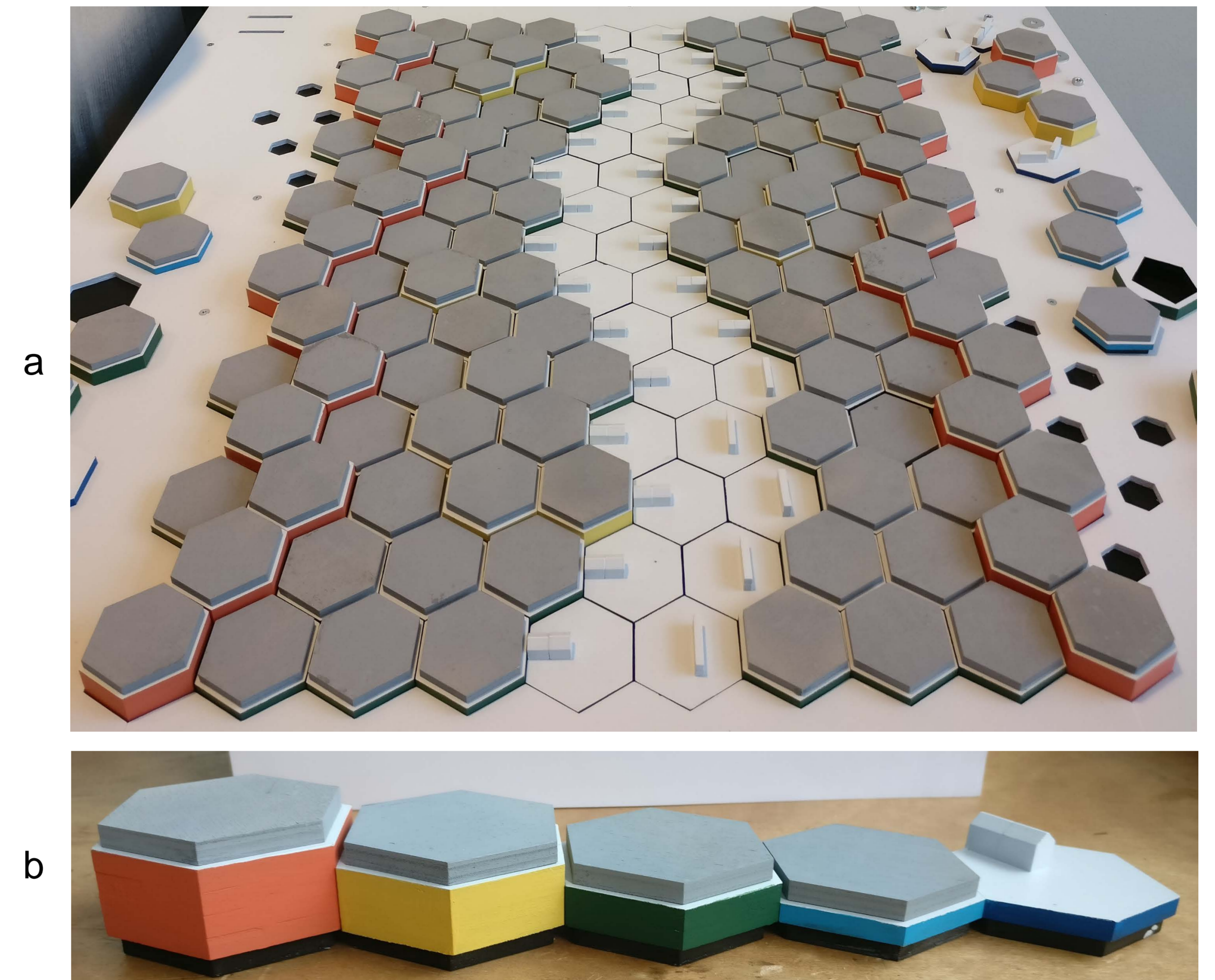
Fig 1. (a) Physical game board, including a main channel with groynes and longitudinal training dams, dikes on the west and east side, and floodplains with varying land uses. (b) Hexagon shaped game pieces representing different heights following a color scheme.
